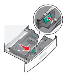
3 Squeeze and then slide the length guide to the correct position for the paper size you are loading.
